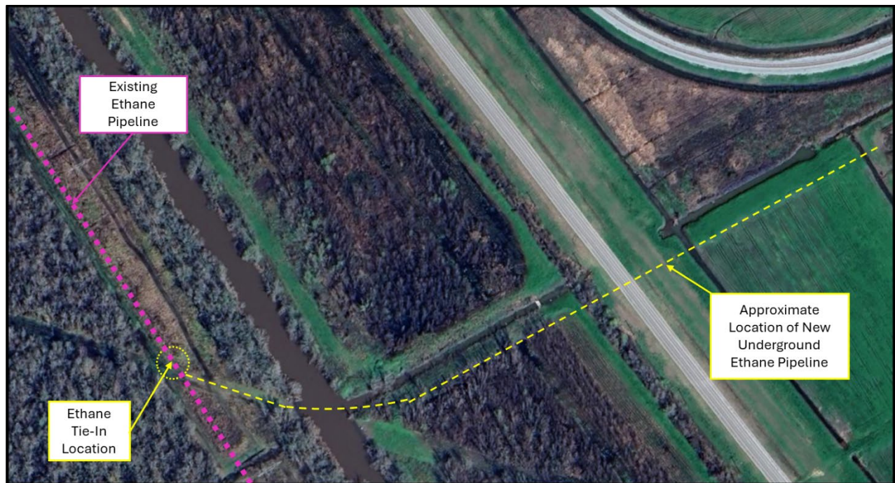
Image 3 – Tie-In Location to Existing Ethane Pipeline in Existing Right of Way Corridors (Google Earth Image)
